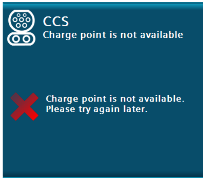
Figure 2-25 Charging point not available using the example of the "CCS" DC charging output
