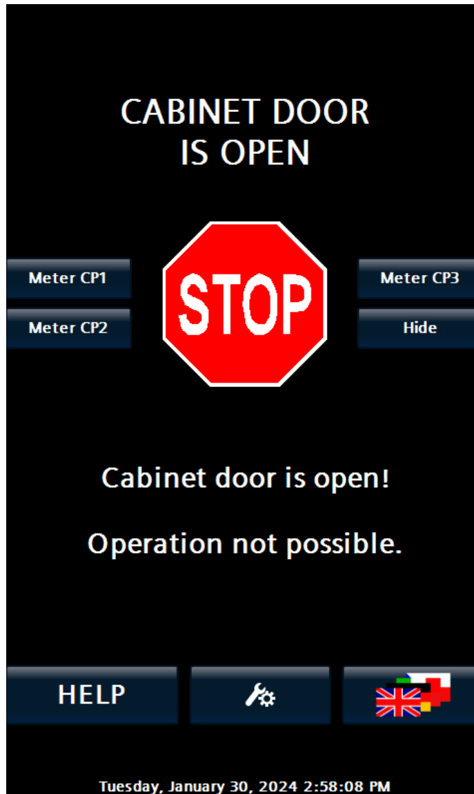
Figure 3-83 Control cabinet door open or not fully closed
