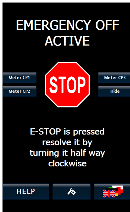
Figure 3-81 Screen "EMERGENCY OFF active"
