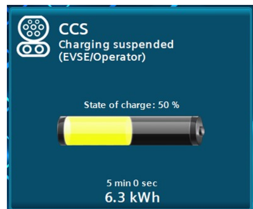
Fig 17: DC charging process "Charging process interrupted by charging station / operator".
